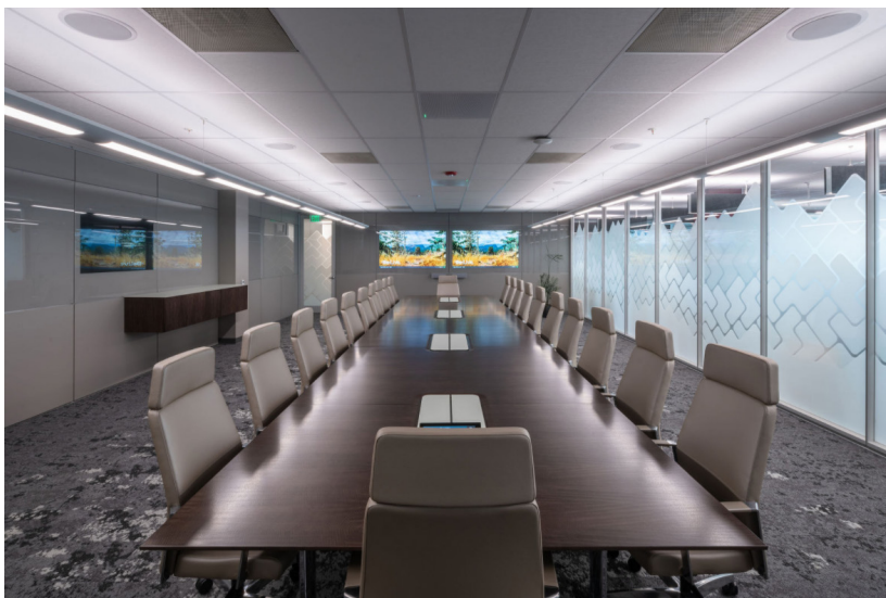
Canvas Credit Union: Prefab solutions include insulated, prefinished solid walls with embedded technology; glass walls with branding/graphics; sliding barn doors; and swing doors.
